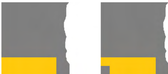
Figure 95 - Cross-sections of leads to QFN components having full lead (left) and lead pullback (right) design.
