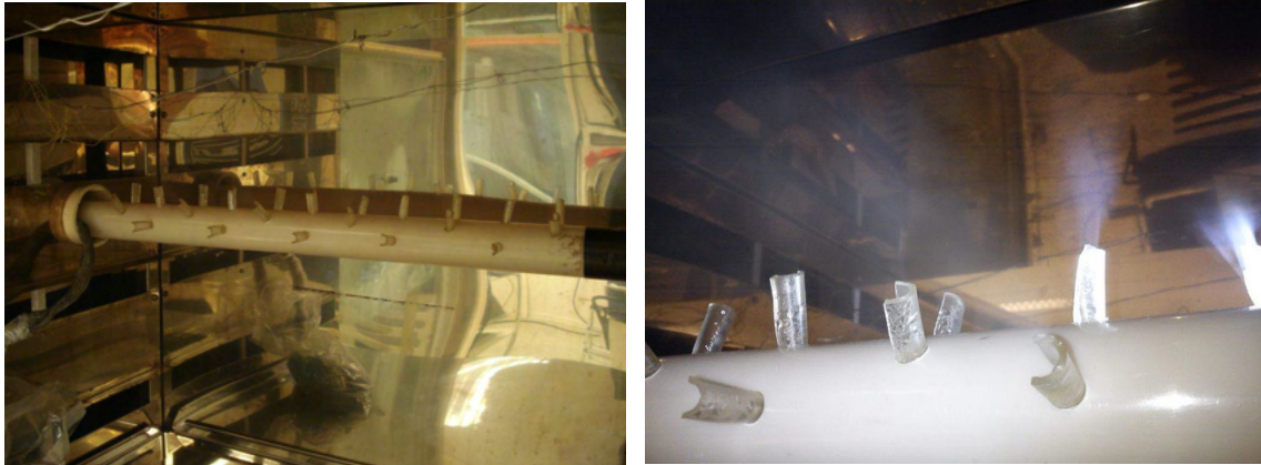
Figure 35 - Photographs showing the tube used for distributing the mist inside the humidity cabinet.
